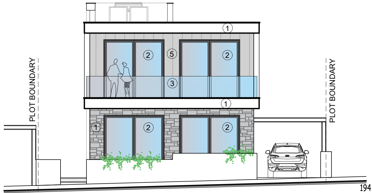
front elevation (south-east)
